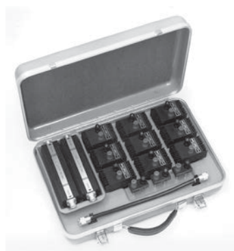
The 5790A is compatible with Fluke A40 and A40A Current Shunts to permit measurements to 20A.
